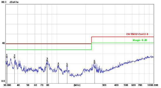
Site LAB Limit: EN 55032 CLASS B Polarization: Vertical
